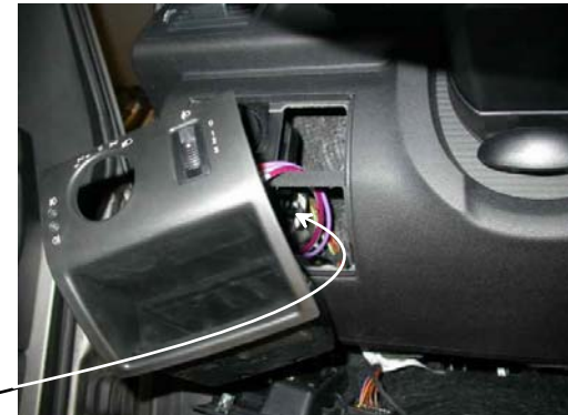
AIR OUTLET PANEL IS FASTENED ONLY WITH CLIPS
