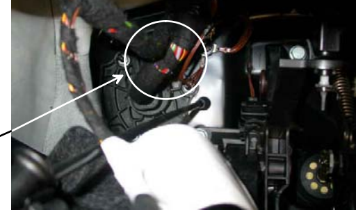
WIRE HARNESS TO/FROM ENGINE DRIVER SIDE
