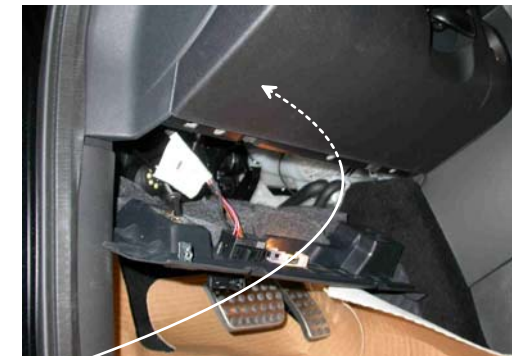
AIR OUTLET PANEL IS FASTENED ONLY WITH CLIPS
