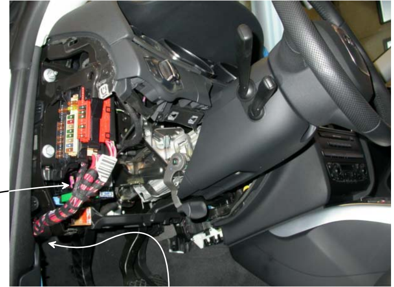
ELECTRONIC CONTROL MODULE LOCATED UNDER DASHBOARD DRIVER SIDE
